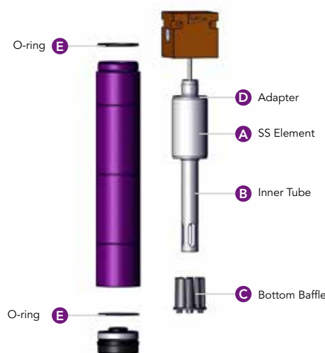
Figure 3 : Water Separator
