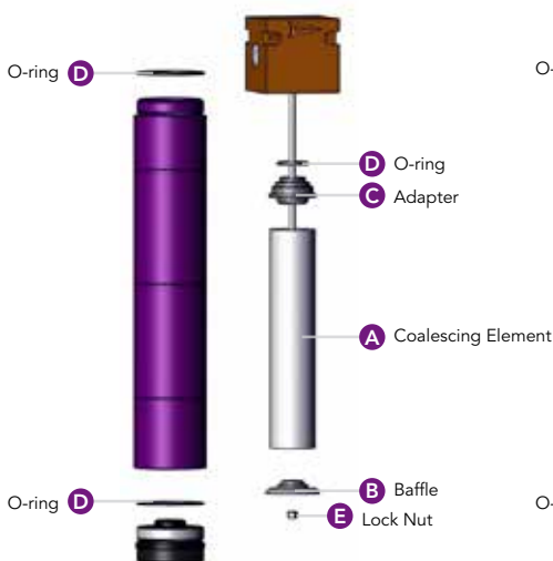
Figure 4 : Oil Coalescing Filter
